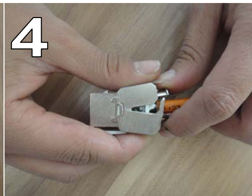
4 Finish the assembly by hand, and cut the excess wires
